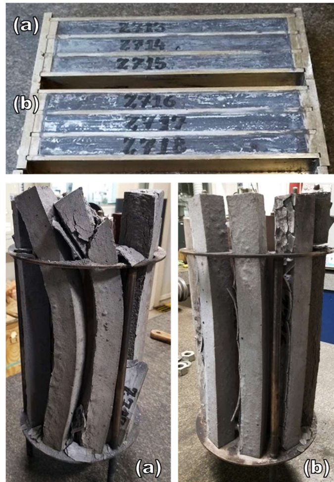
Figure 13. Samples with 90 % cement replacement by volume before and after the soundness test: (a) 80% BOFS-L + 10% BOFS-H; (b) 80% BOFS-L + 10% QIT-H.
