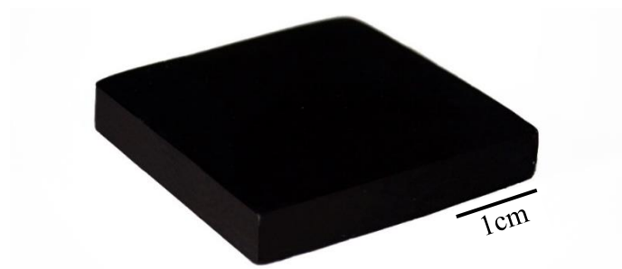
Figure 2.6. Macroscopic appearance of fired CT-3 tiles, showing the typical dark brown luster.
