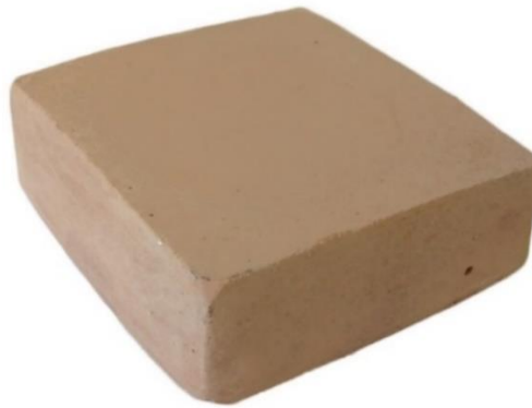
Fig. 4.2. Sample of the colour layer with IOT as aggregate, for pigment evaluation.
