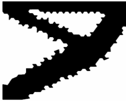
Figura 3.22 – Viga curta bi-apoiada – MEC - \bar{A} = 40\% A Marczak (2006).
