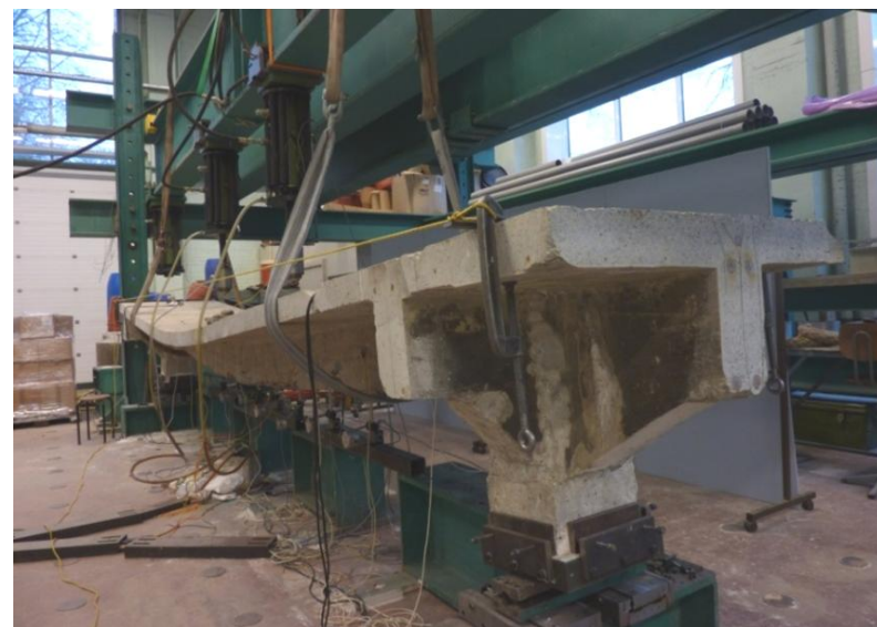
Testing to failure of an early reinforced concrete beam (1904) - span 6 m
