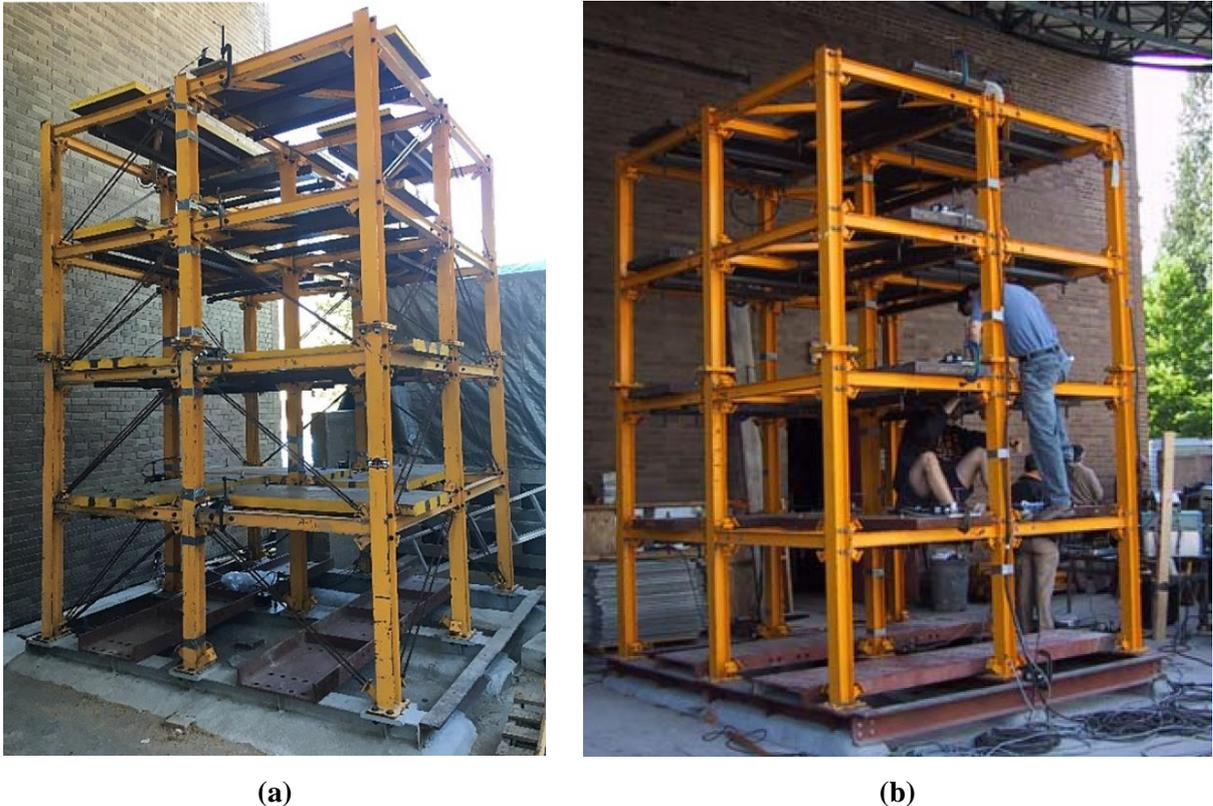
**Fig. 5.6** Tested frame structure: (a) braced and (b) unbraced.
