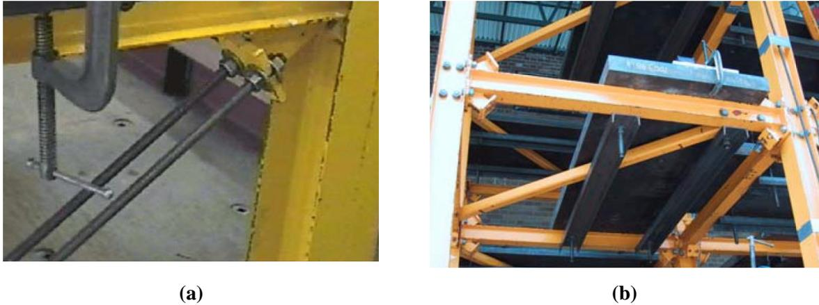
**Fig. 5.7** Zoom at (a) bracing and (b) mass placement.
