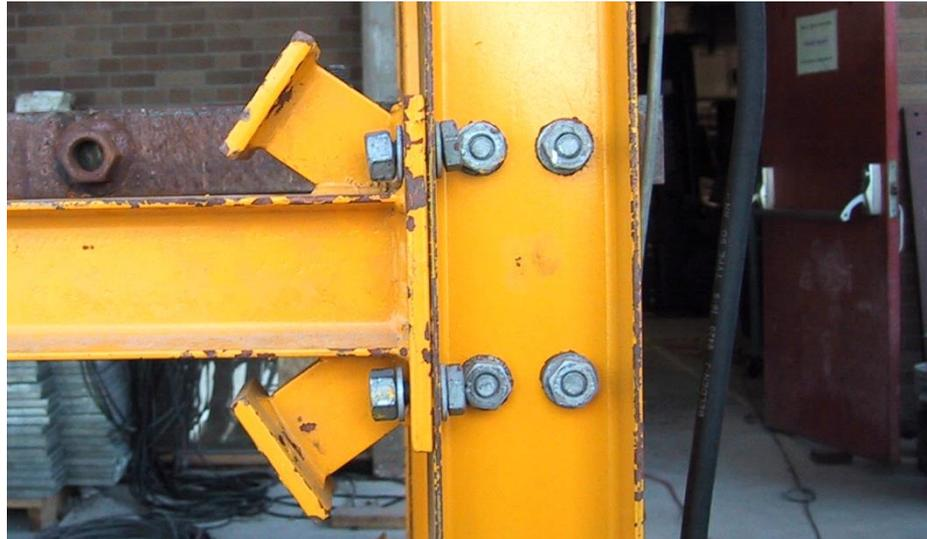
**Fig. 5.11** Photograph showing typical loosened bolts at beam-column connection (cases 8 and 9).
