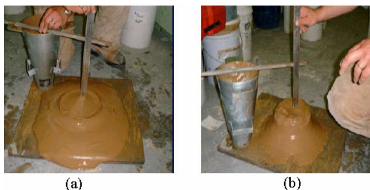
Figura 2. 6– (a) Slump de pasta 250 mm, e (b) Slump de pasta 175mm (Grabinsky et al. 2002)
